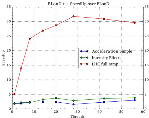
Each line corresponds to a test-case of different complexity level. The top Speed-Up achieved in the two less complex test-cases is up to 3.0X and 3.9X respectively. However, the results are different in the most complex case, demonstrating a maximum Speed-Up of 31.8X.
