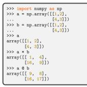
$$\begin{bmatrix} a_{11} & a_{12} \\ a_{21} & a_{22} \end{bmatrix} * \begin{bmatrix} b_{11} & b_{12} \\ b_{21} & b_{22} \end{bmatrix} = \begin{bmatrix} a_{11} * b_{11} & a_{12} * b_{12} \\ a_{21} * b_{21} & a_{22} * b_{22} \end{bmatrix}$$
