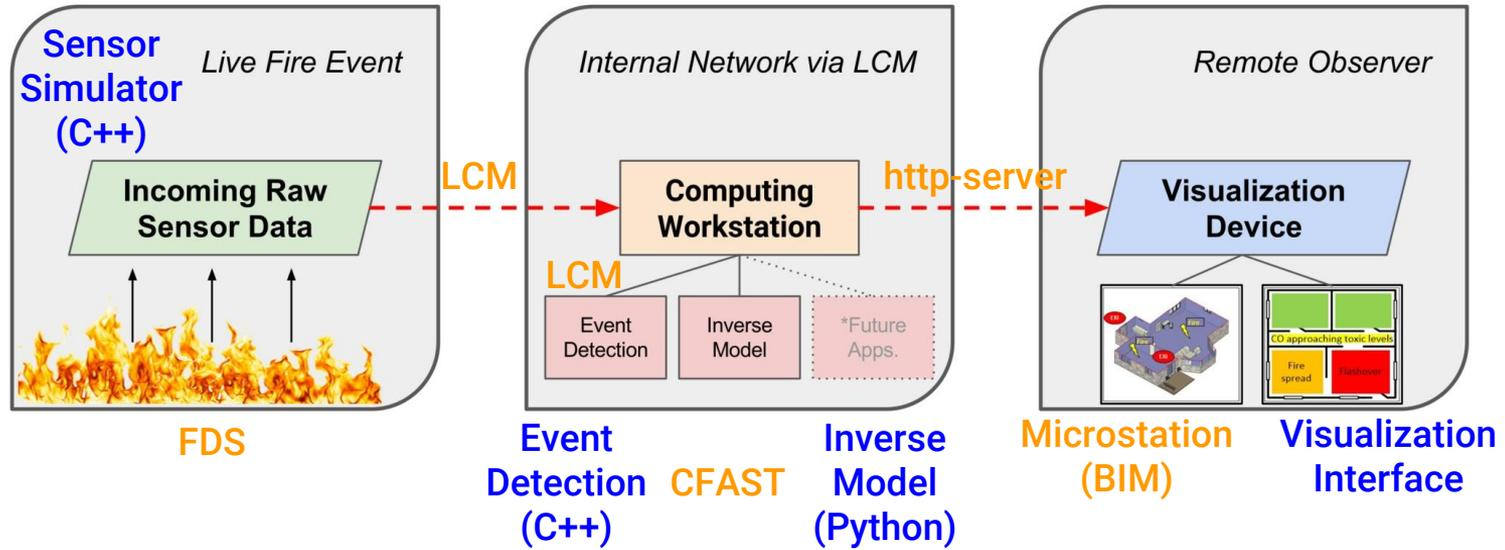
**Main Program (Python):** Facilitates data transfer via LCM and handles the main event loop for simulating the real-time fire scenario.
