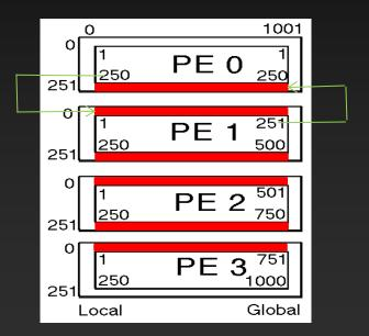
The program has a local view of data. The programmer has to have a global view of data. The ghost cells don't exist in the global dataset. They are only copies from the "real" data in the adjacent PE.
