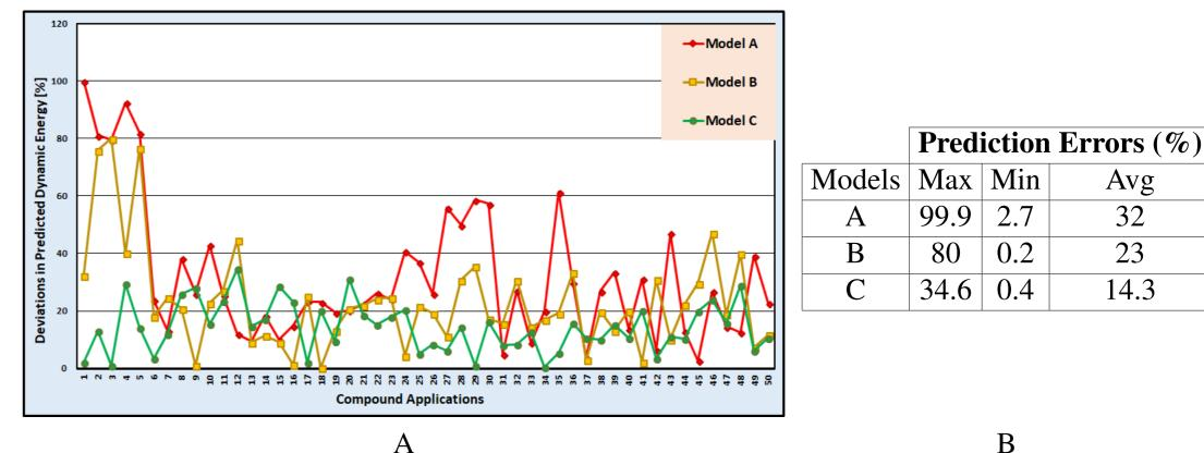
(A) Non-additivity of PMCs effecting the prediction accuracy of models. Model A uses 6 well-known PMCs, Model B using highly correlated PMCs and Model C using one highly additive PMC. (B) Models' prediction errors. Model training data set = 277 points. Model testing data set = 50 points
